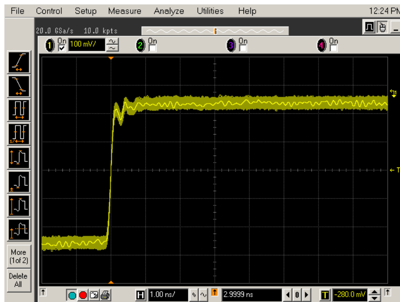
Figure 20 Good Connection Waveform Example
